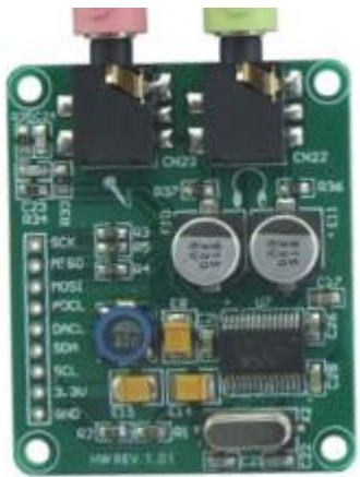
Figure 4 AUDIO CODEC Proto by MikroElektronika one of the two integrated circuit systems being used for analog to digital conversion.
